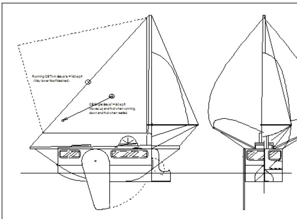
You'll probably notice some funny things in the drawing. Yes, the mast backstay *is* spread by the mizzen boom and swings along with it. The mizzen is used for beating or riding. When running (most of the time), it's to be (double)sheeted amid-ships. While the mast is on the centerline, the sprit and boomkin are not. The stay system isn't optimal, but improves on *no* stay, is easily and quickly dismantled, and keeps the number of parts low by making them wear more hats.
