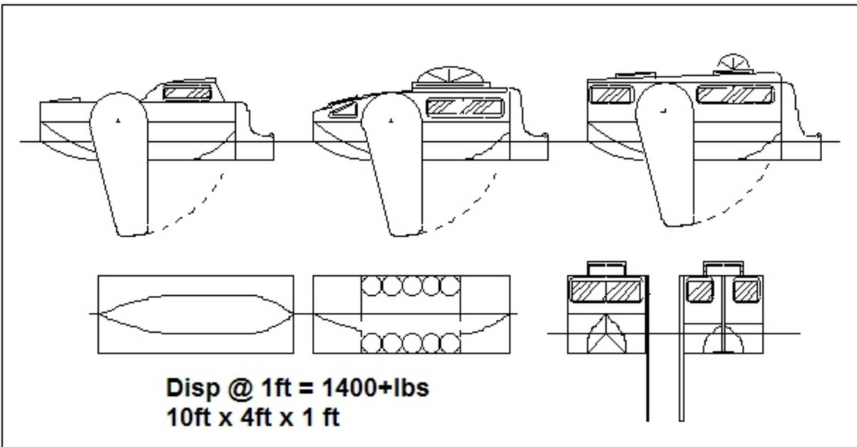
The hull is essentially a barge, which racks up maximum displacement and interior volume for any given dimensions. Or, from another direction, the beam can be kept slender and draft shallow and still achieve reasonable displacement. A step keel has been added to further increase displacement. Beam could be increased, if necessary, for yet more.
