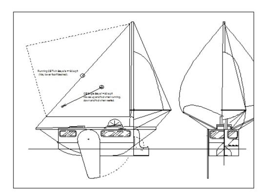
You'll probably notice some funny things in the drawing. Yes, the mast backstay *is* spread by the mizzen boom and swings along with it. The mizzen is used for beating or riding. When running (most of the time), it's to be (double)sheeted amid-ships. While the mast is on the centerline, the sprit and boomkin are not. The stay system isn't optimal, but improves on *no* stay, is easily and quickly dismounted, and keeps the number of parts low by making them wear more hats.
