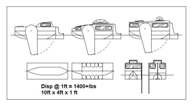
The hull is essentially a barge, which racks up maximum displacement and interior volume for any given dimensions. Or, from another direction, the beam can be kept slender and draft shallow and still achieve reasonable displacement. A step keel has been added to further increase displacement. Beam could be increased, if necessary, for yet more.
