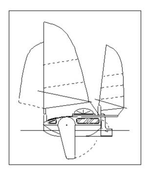
This is a much simpler rig, with minimal control lines. The entire foot of the main can be reached from the hatches for control or reefing.
